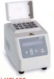
Mini Dry bath is portable, compact and convenient. It is useful for rapid and uniform heating of biological samples, in applications like preservation and denaturation of nucleic acids and proteins and many other applications.
